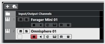
**Step 2:** On the "Midi From" drop down on your instrument track, change from "All Ins" and select the MIDI track that Forager Mini is on.
