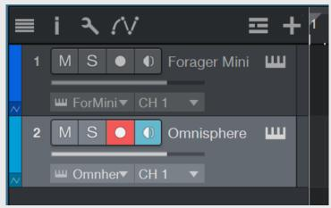
**Step 2:** On your instrument's track, expand the height of the track to make the Input selector visible.
